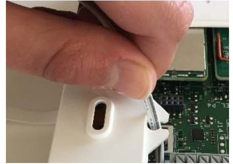
Insert the wire into the strain-relief
