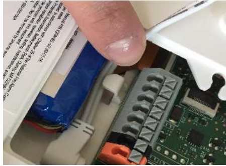
Route the wire behind the retainer clip
